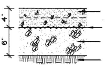
STONEDUST & ORGANIC BINDER 15# BINDER/TON AGGREGATE PLACED IN TWO 2-INCH LIFTS
